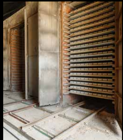
Hand-moulded bricks dry from the inside out in the drying chambers
