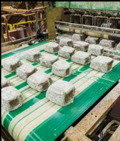
Pressed clay balls, ready for moulding
